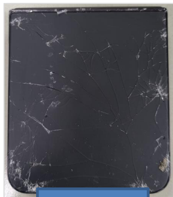
Rear Glass cracked
