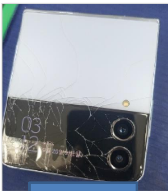
Front Glass cracked
